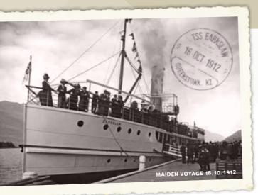
Named after Mount Earnslaw (the highest peak in the region), she is 168 feet in length, 24 feet across the beam and weighs 330 tonnes. Originally built by J McGregor & Co in Dunedin at a cost of £20,850, the TSS Earnslaw was dismantled and transported by rail to Kingston at the lake's southern tip for reassembly and launching.
